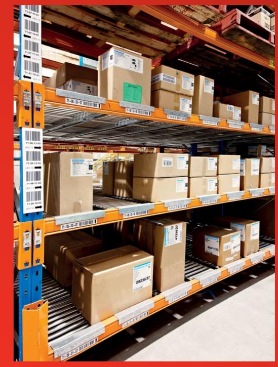
Roller Flo provides a robust carton live storage solution. It provides an adaptable alternative to pallet or split case picking, depending on your requirements.
