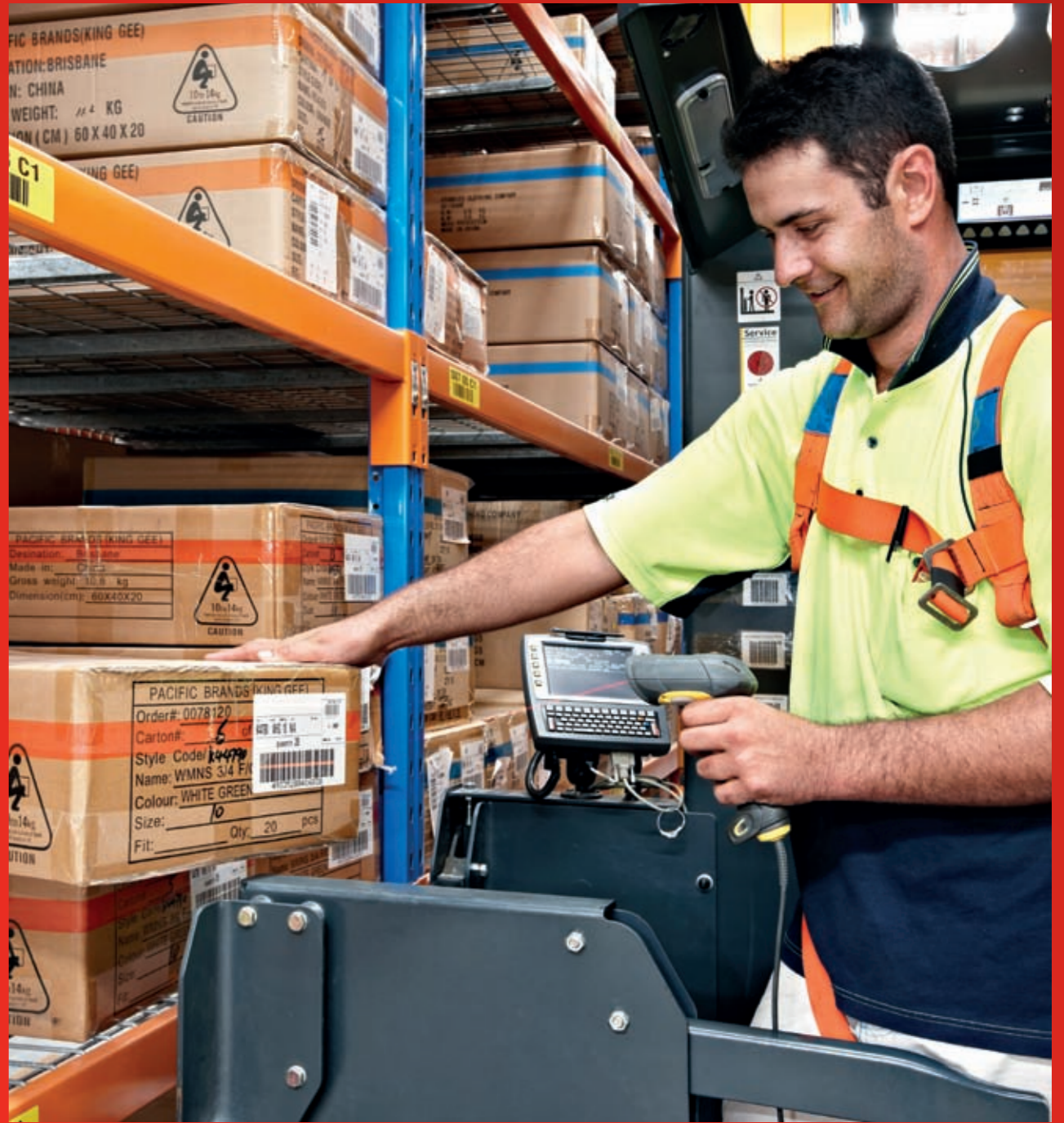
The system is served by forklifts with elevating operator cabins. The operator hand picks.
