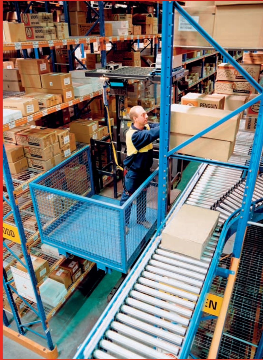
Mesh decks provide strength while allowing airflow and light filtration.
