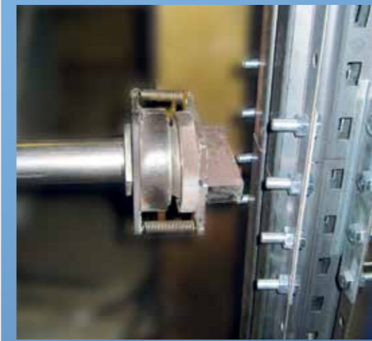
TEST: UPRIGHT SPLICE.
