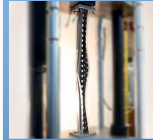
TEST: UPRIGHT LONG COLUMN.
