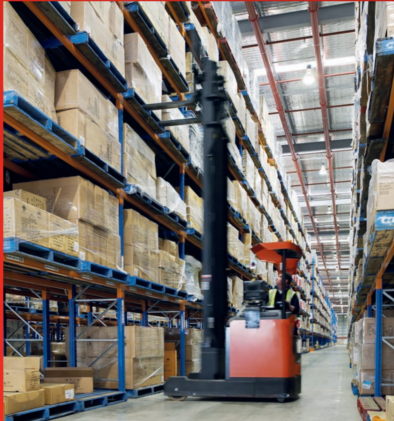
Pallets can be located, accessed and moved individually, allowing rapid handling of almost all types of palletised goods.
